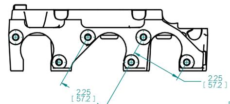
BRACKET CONNECTION REQUIRES 2 BOLTS. USE WIDEST SPREAD AVAILABLE PER PAD ANGLE DESIRED. 1.0" BOLT SPREAD MINIMUM
